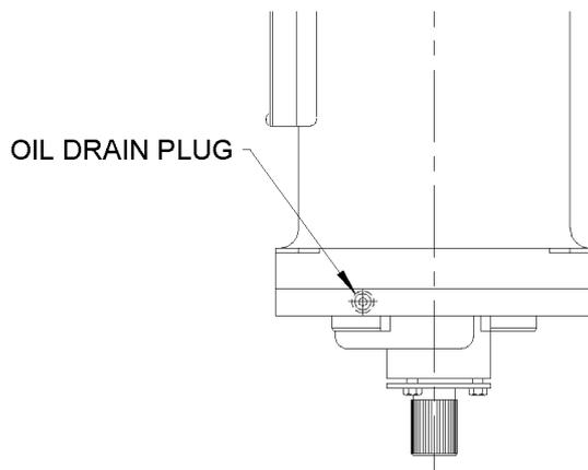
Figure 4.3 Oil Drain Plug
