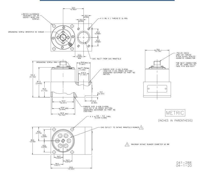
Figure 1-1b. SOGAV 43 Outline Drawing (MS Connector)
