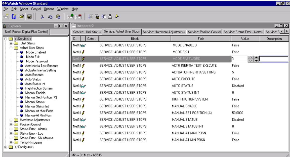
Figure 9-6. Service Mode: Adjust User Stops
