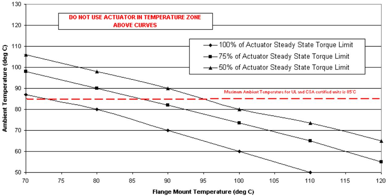
Figure 2-3. Flange Mount Actuator Selection Guidelines
