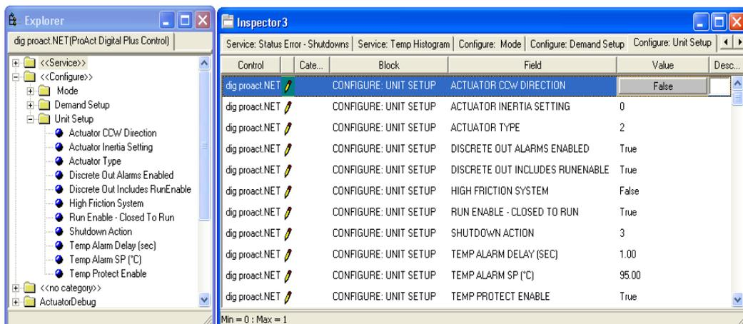
Figure 9-2. Configure Mode: Unit Setup
