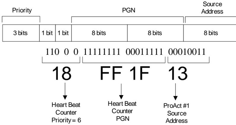
Figure 7-1. Typical Arbitration Field Example
