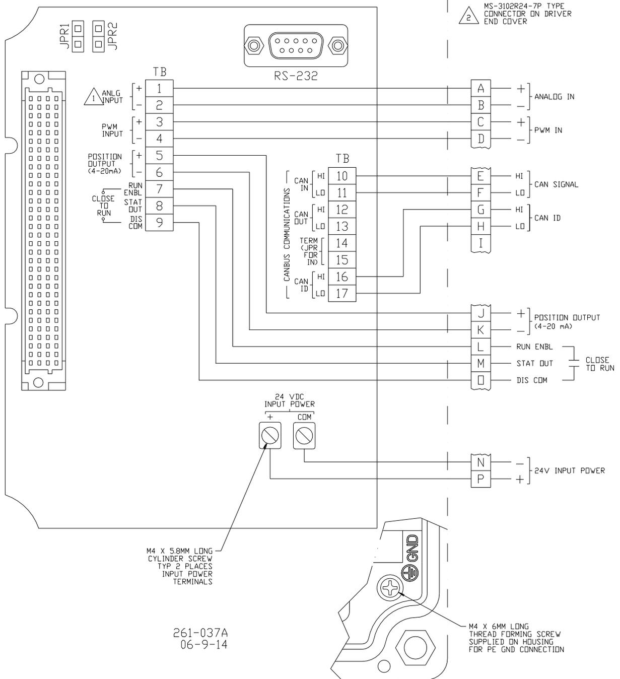
Figure 3-1c. Control Wiring Diagram (Digital Plus)
