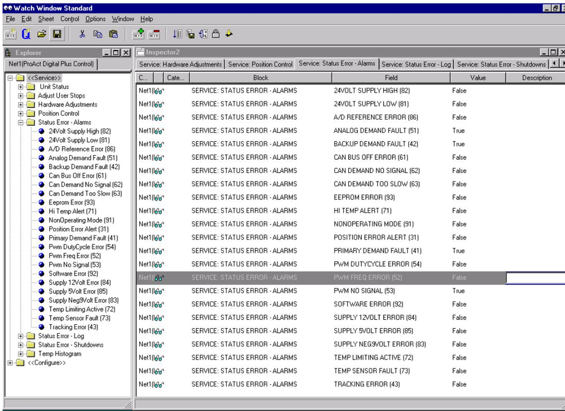
Figure 9-12. Service Mode: Status Error Alarms
