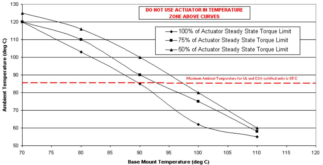
Figure 2-2. Base Mount Actuator Selection Guidelines
