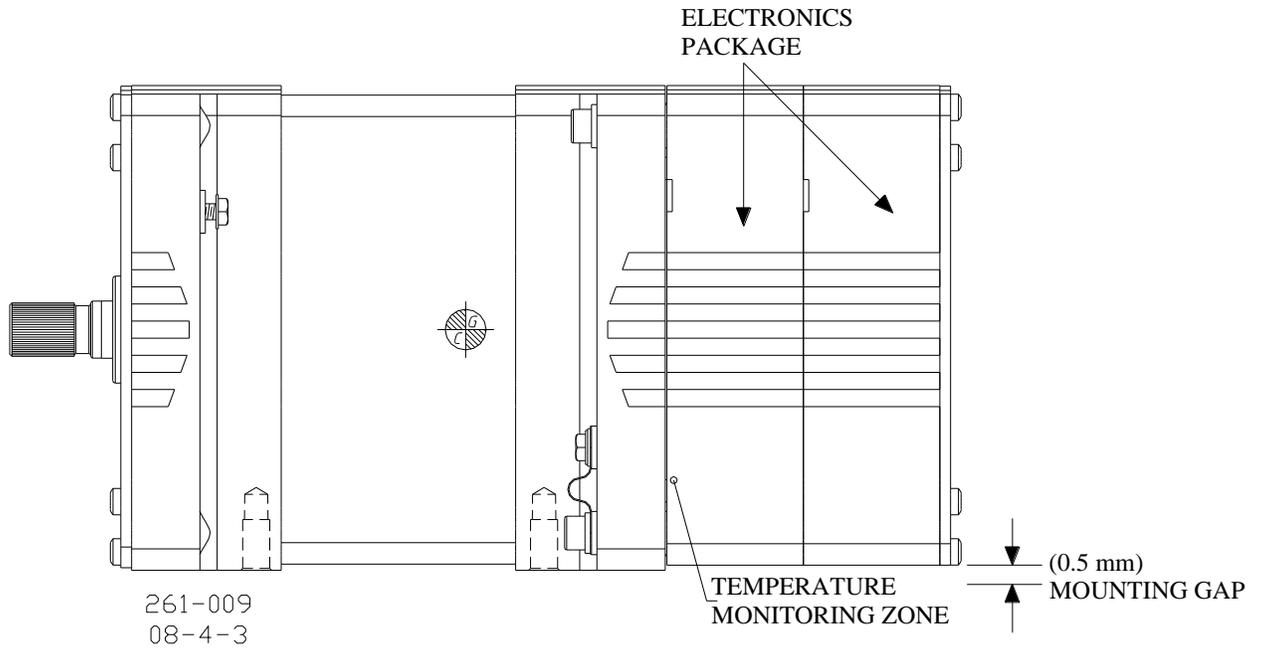
Figure 2-1. Temperature Monitoring Zone (model III shown)
