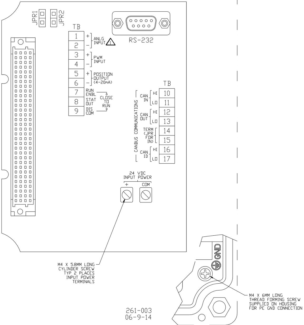
Figure 3-1a. Control Wiring Diagram (blank cover)
