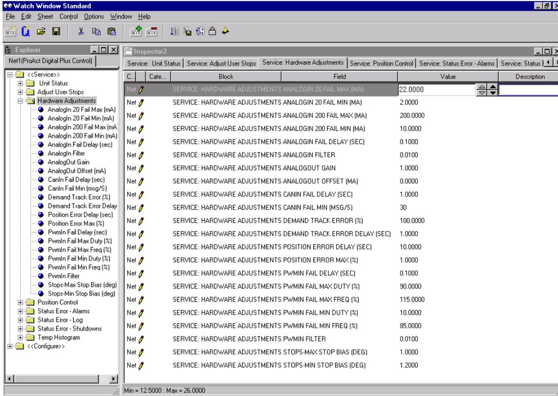
Figure 9-9. Service Mode: Hardware Adjustments
