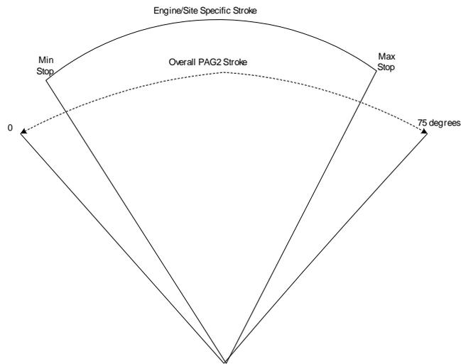
Figure 9-4. Min/Max Stops Relative to the Overall Travel
