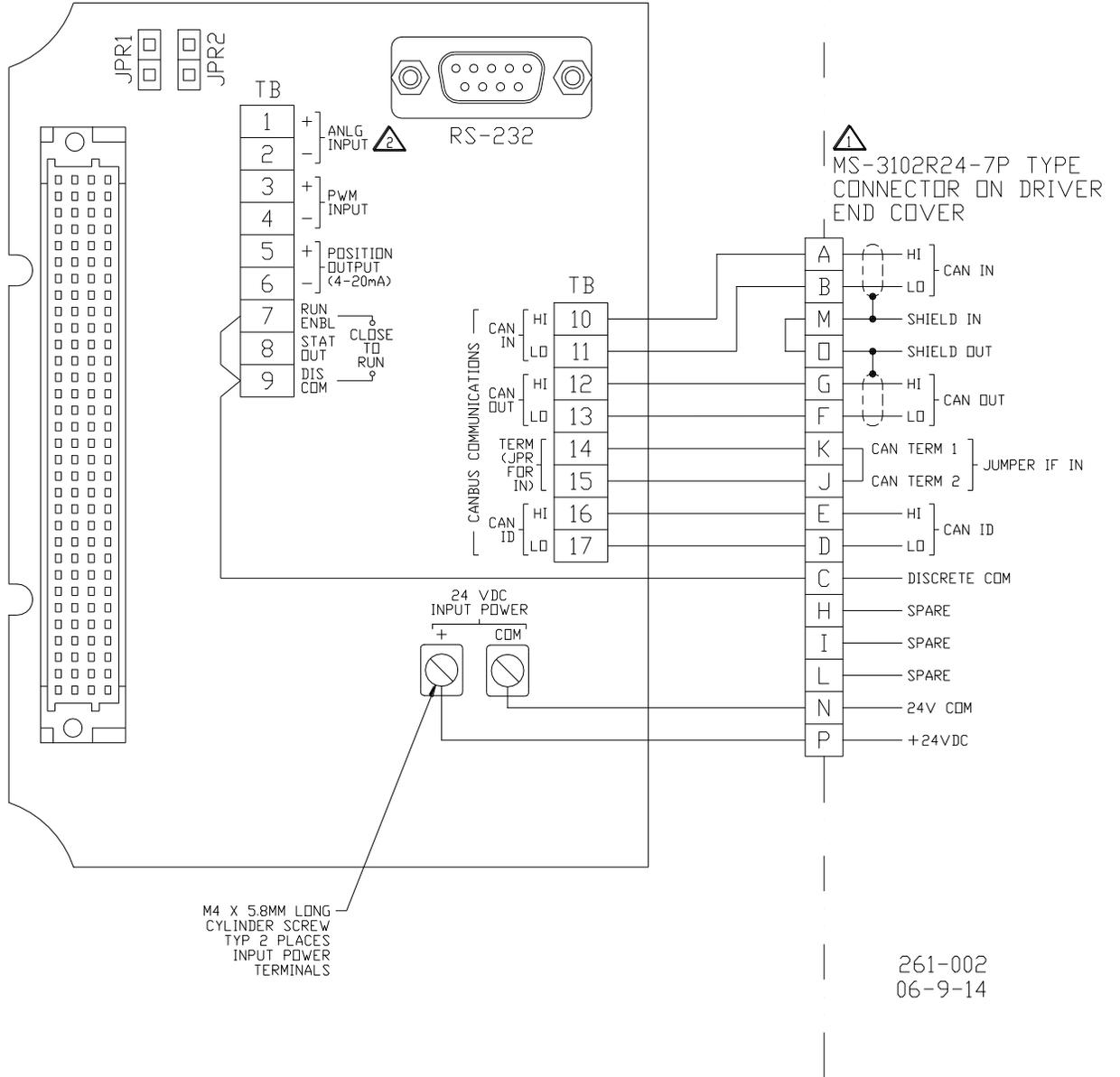
Figure 3-1b. Control Wiring Diagram (CAN only)
