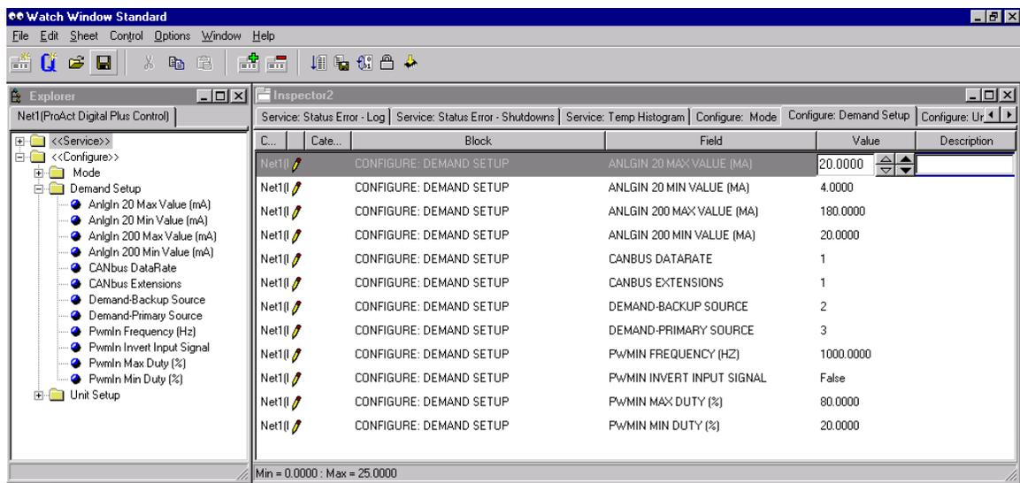
Figure 9-3. Configure Mode: Demand Setup
