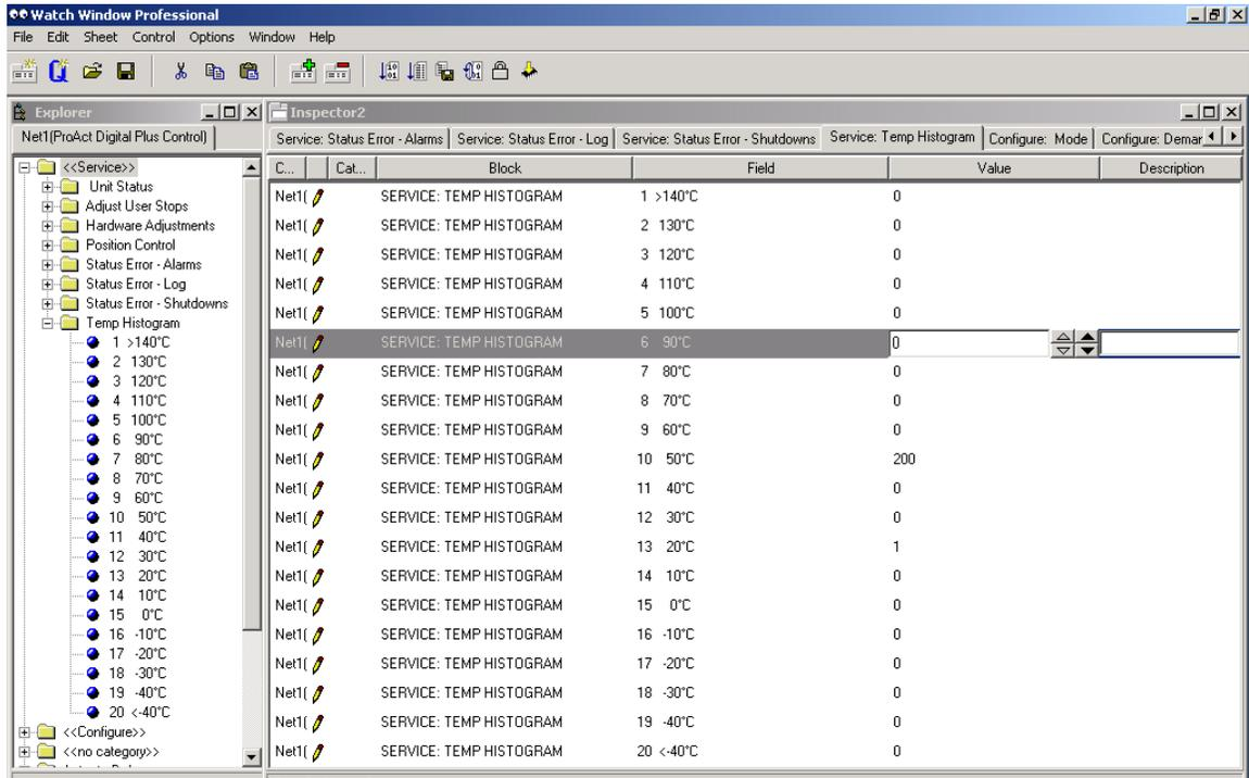
Figure 9-16. Service Mode: Temperature Histogram
