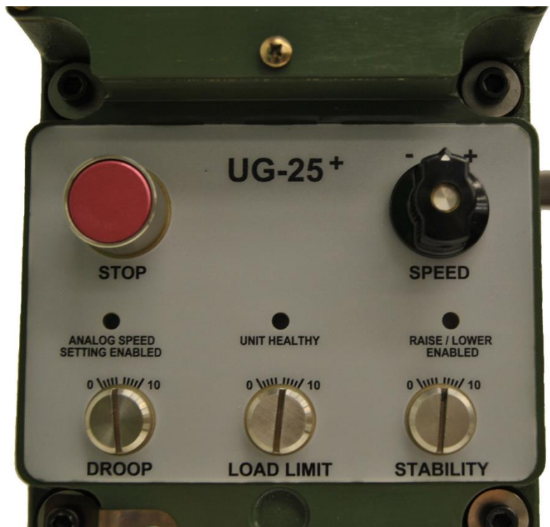
Figure 4-1. UG-25+ Governor Front Panel Overview
