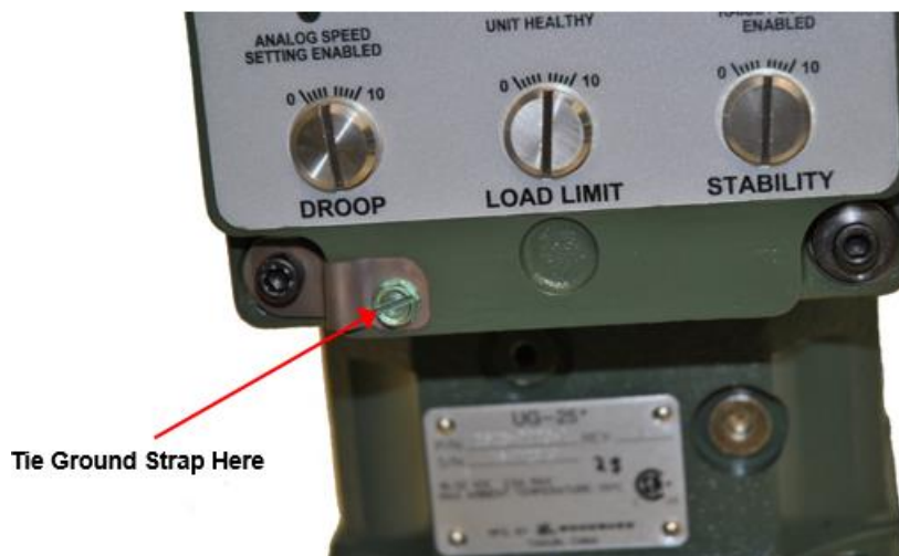
Figure 3-1. Location of Ground Strap
