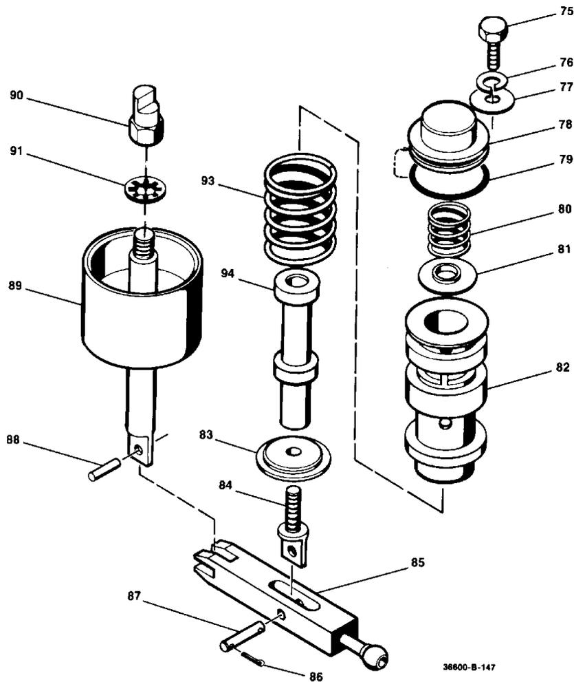
Figure 6-2. Parts for Power Piston Assembly and Pilot Valve Assembly
