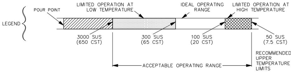
Figure 2-1. Viscosity and Operating Temperature of Oils
