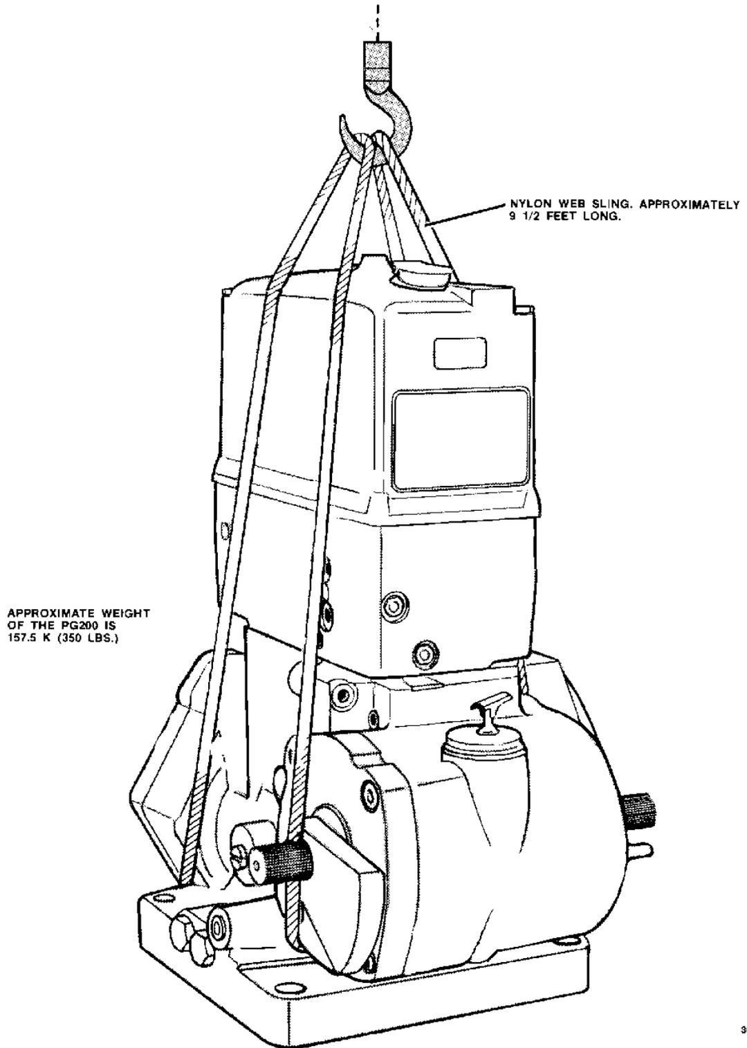
Figure 1-2. Lifting Sling for PG-200/300 Governor
