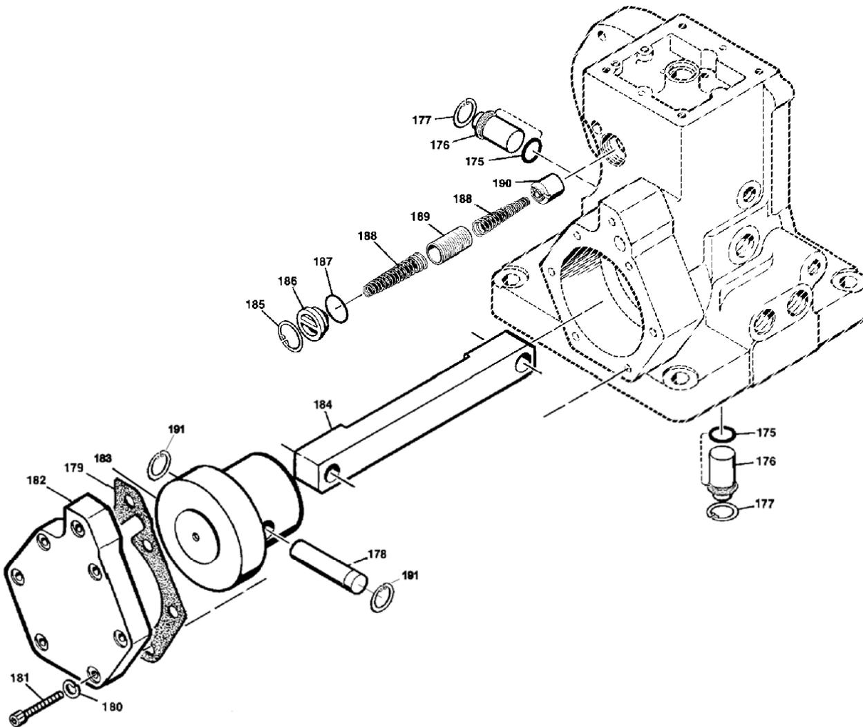
Figure 6-4. Parts for Servo Assembly
