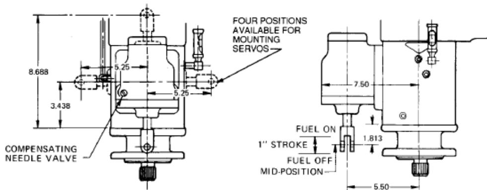
**29/58 ft-lb Differential Power Servo (linear output)**
