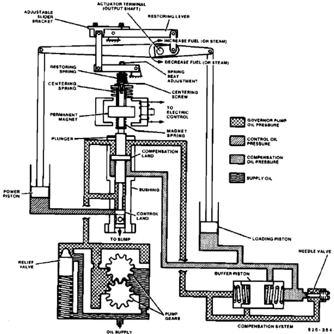
Figure 1-2. EG-3PC Schematic
