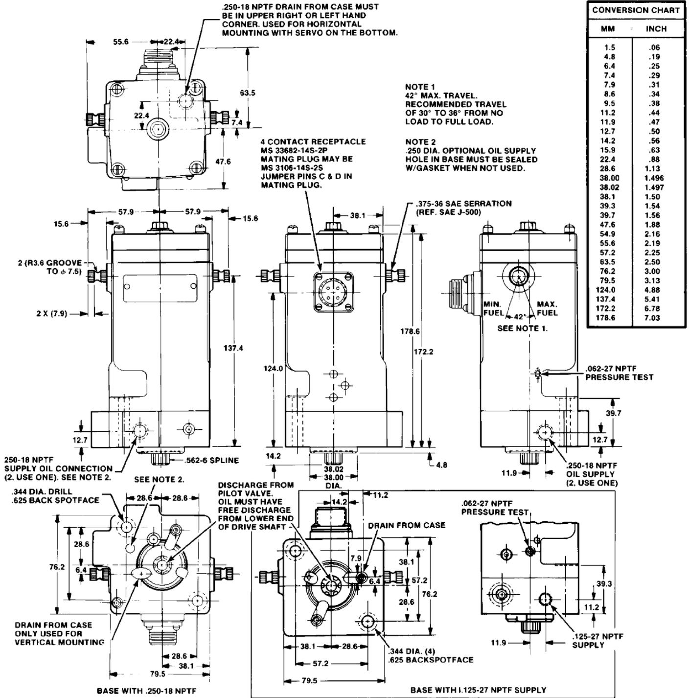
Figure 4-5. Outline Drawing (EG-3P with Oil Pump)
