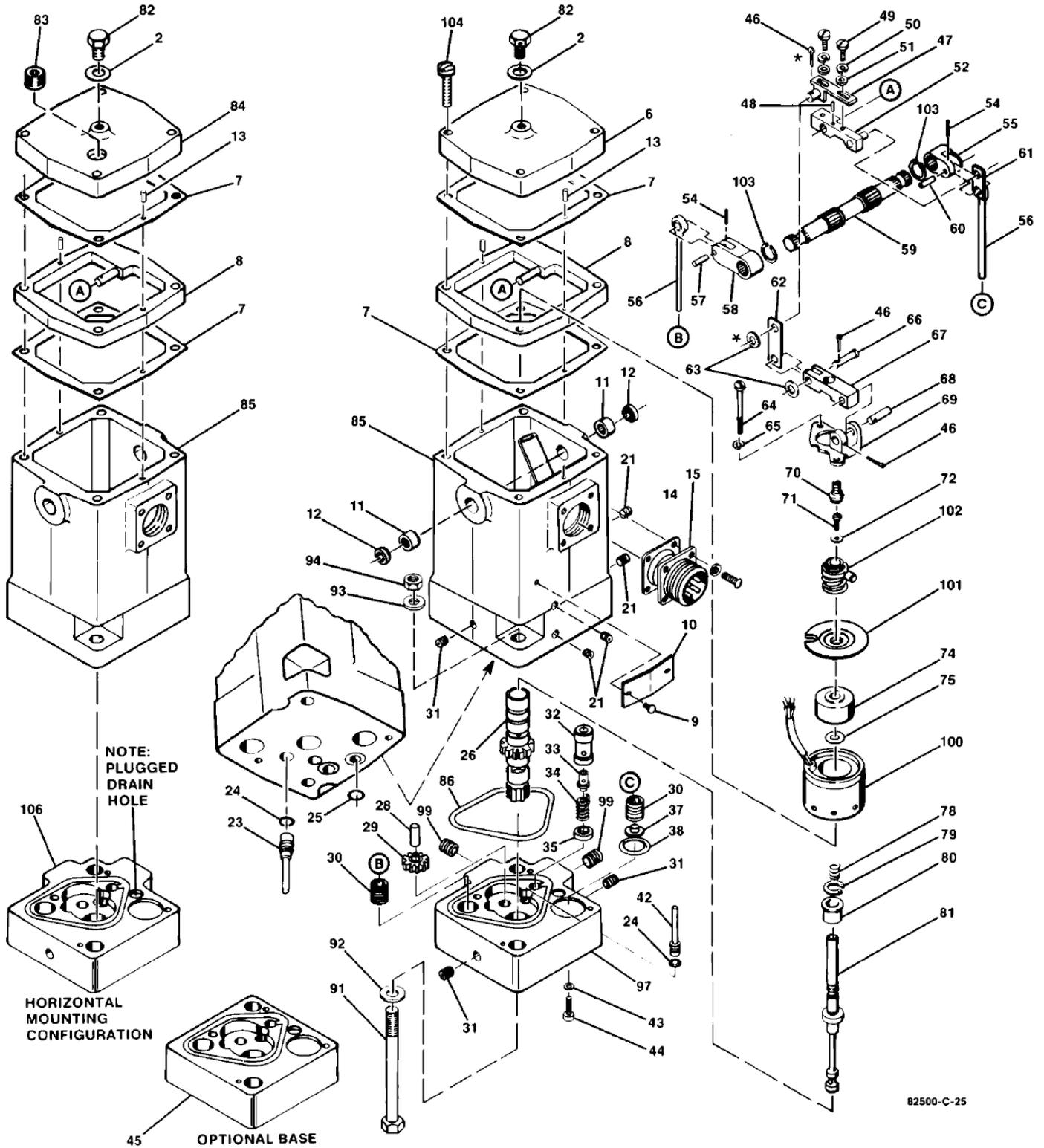
Figure 4-1a. Exploded View (EG-3P with Gear Pump)
