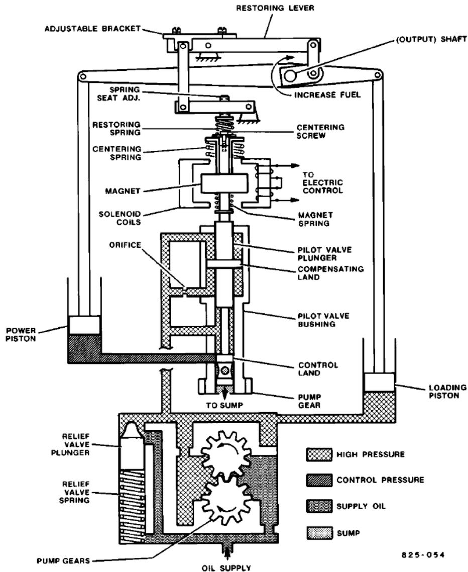
Figure 1-1. EG-3P Schematic
