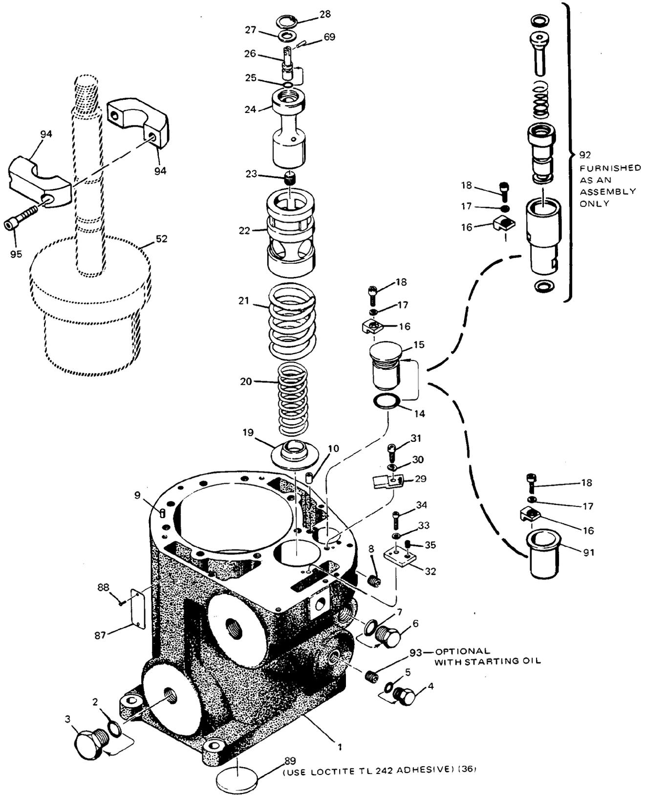
Figure 5-1a. Exploded View, Mechanical Input-Hydraulic Amplifier
