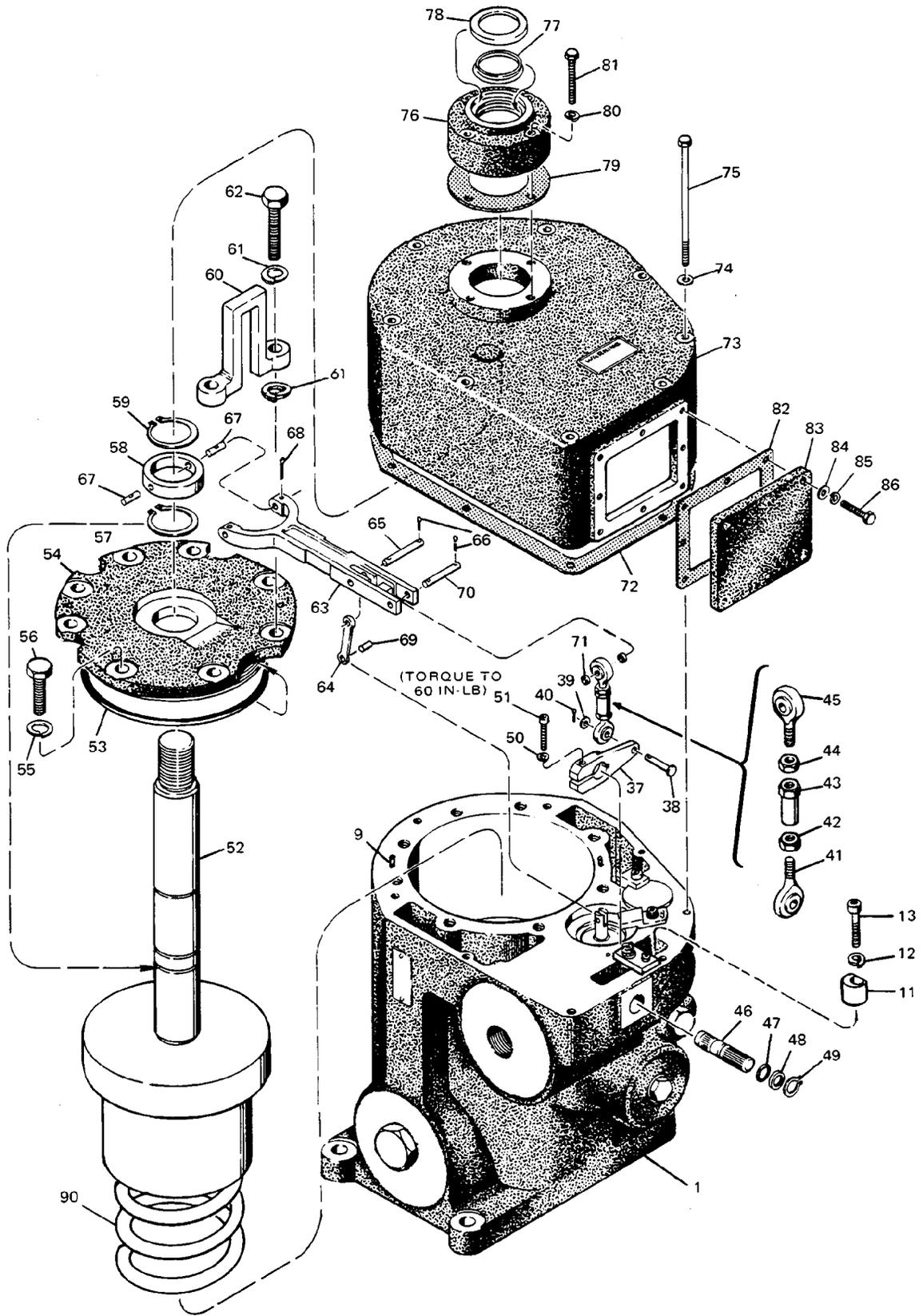
Figure 5-1b. Exploded View, Mechanical Input-Hydraulic Amplifier
