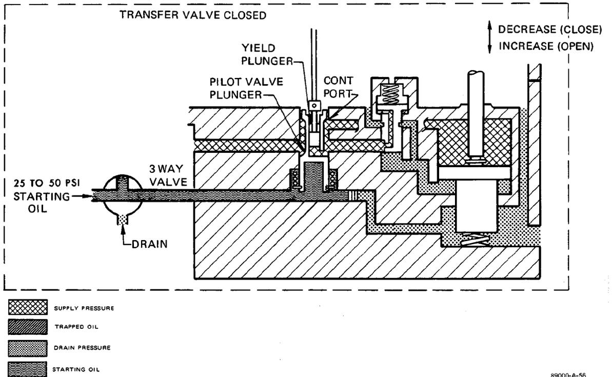
Figure 3-2. Schematic of Mechanical-Hydraulic Amplifier with Yield Plunger and Transfer Valve Closed
