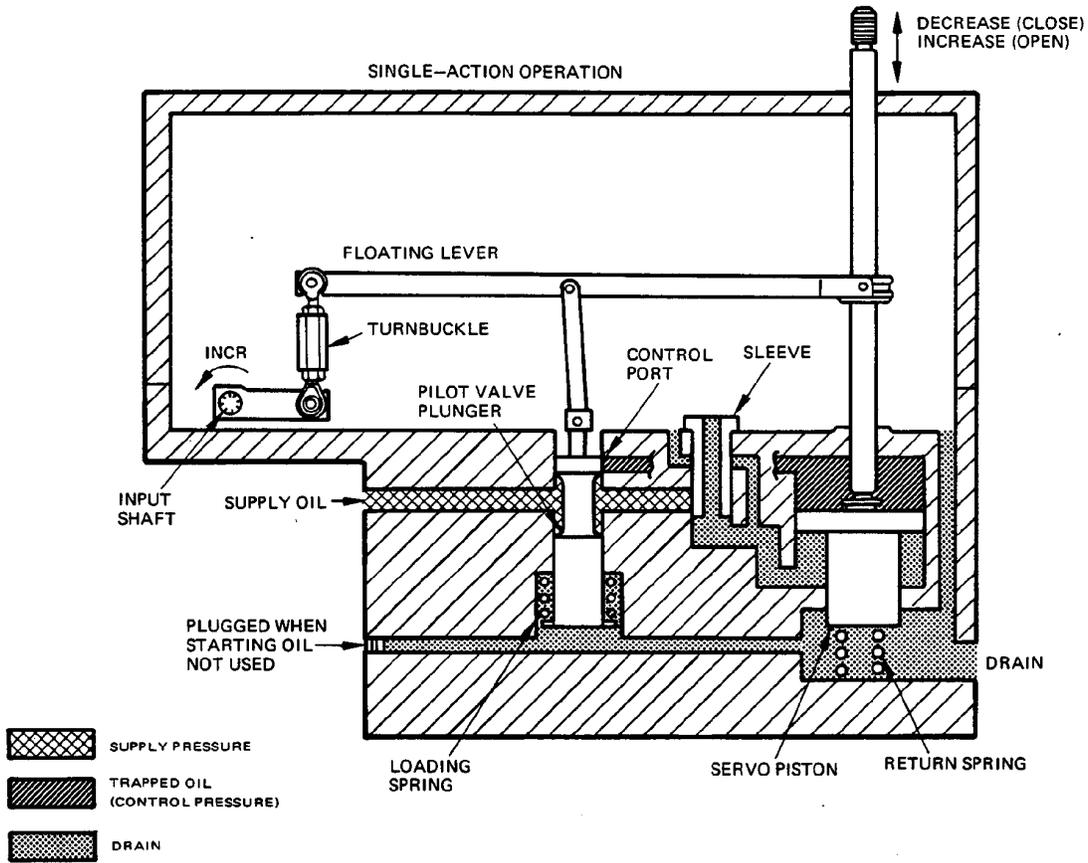
Figure 3-3. Schematic of Mechanical Input Hydraulic Amplifier with Sleeve
