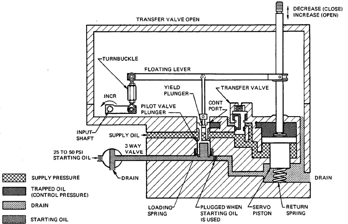
Figure 3-1. Schematic of Mechanical-Hydraulic Amplifier with Transfer Valve Open
