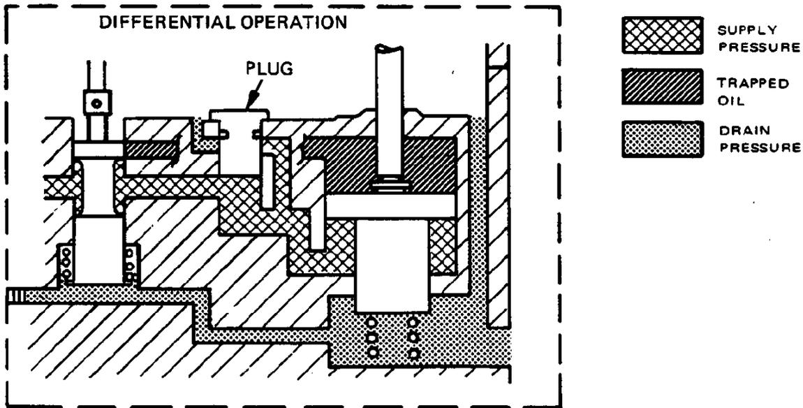
Figure 3-4. Schematic of Mechanical Input Hydraulic Amplifier with Plug
